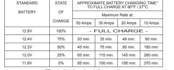
\*Charging time depends on battery capacity, condition, age, temperature and efficiency of charger
